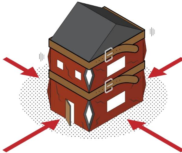
*Figure 1. A damaged building during an earthquake can be held together at floor and roof level by tie or ring beams which function like strong belts.*
